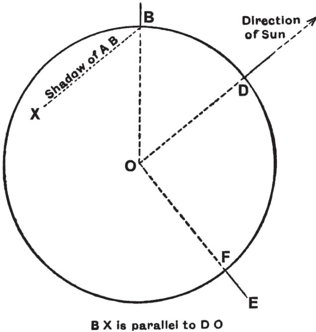
is vertical. Show that a pencil erected at F ( $90^\circ$  from D) throws a shadow on the line which represents the ground. F then represents a place where the sun's altitude is  $0^\circ$ .
