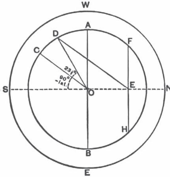
right angles to SN. OC is drawn at an angle to SN equal to  $90^\circ$  diminished by the latitude of the place. COD is  $23\frac{1}{2}^\circ$ . DE is drawn parallel to CO. Through E is drawn FH parallel to AB. FH is the second slit. The third is drawn the same distance to the left of AB that FH is to the right.
