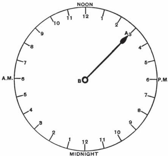
describes a circle in twelve hours, i.e. half the time that the sun takes to complete its circle. As the watch hand moves twice as quickly, we can use the above cardboard dial but we must halve the angle.
